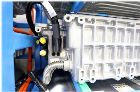
Fig.: Integrated exhaust air duct
